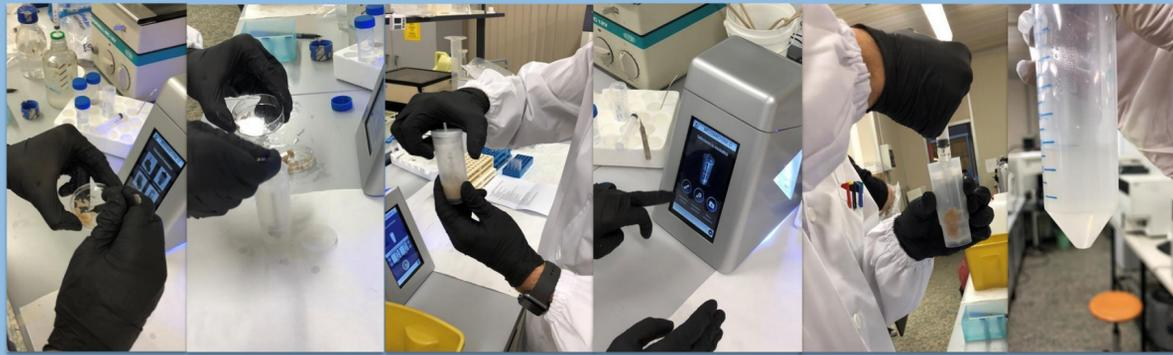
Fig. 1 Photographs of the homogenization procedure with Medimachine II.
